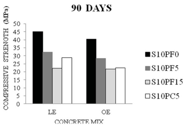
Fig 3. The results of compressive strength of specimens
