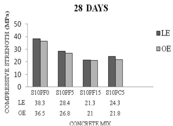
Fig 10. The results of curing conditions on compressive strength
