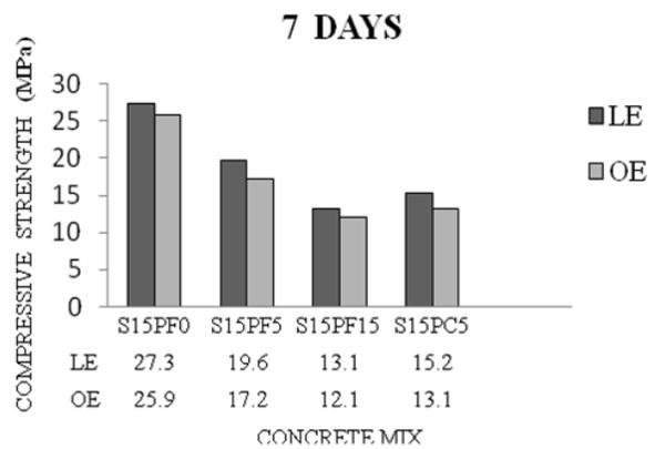
Fig 12. The results of curing conditions on compressive strength
