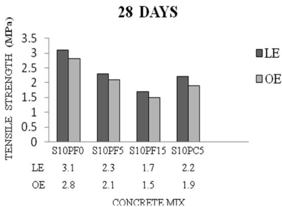
**Fig 15. The results of curing conditions on tensile strength**
