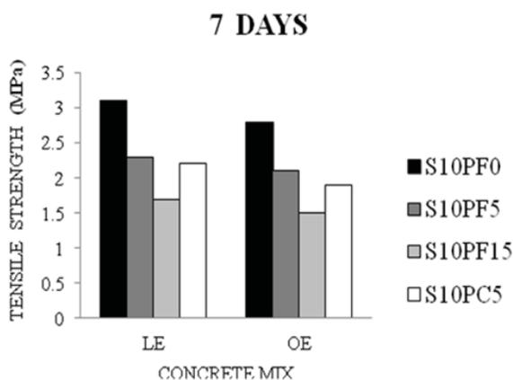
Fig 7. The results of tensile strength of specimens
