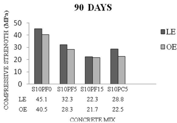
Fig 11. The results of curing conditions on compressive strength
