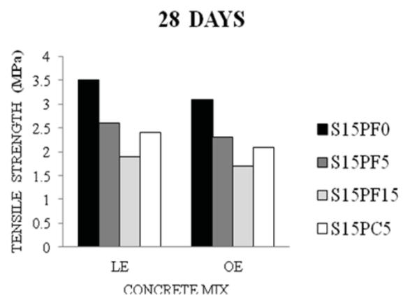
Fig 8. The results of tensile strength of specimens
