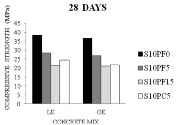
Fig 2. The results of compressive strength of specimens
