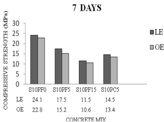
Fig 9. The results of curing conditions on compressive strength
