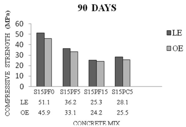
Fig 14. The results of curing conditions on compressive strength
