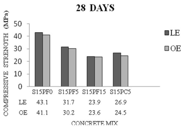
Fig 13. The results of curing conditions on compressive strength
