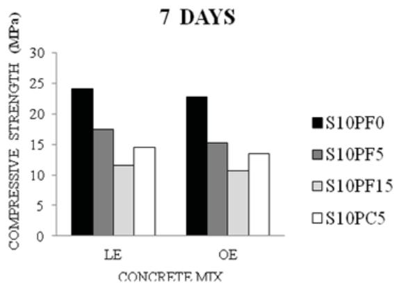
Fig 1. The results of compressive strength of specimens
