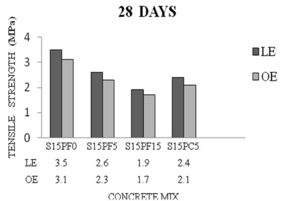
**Fig 16. The results of curing conditions on tensile strength**
