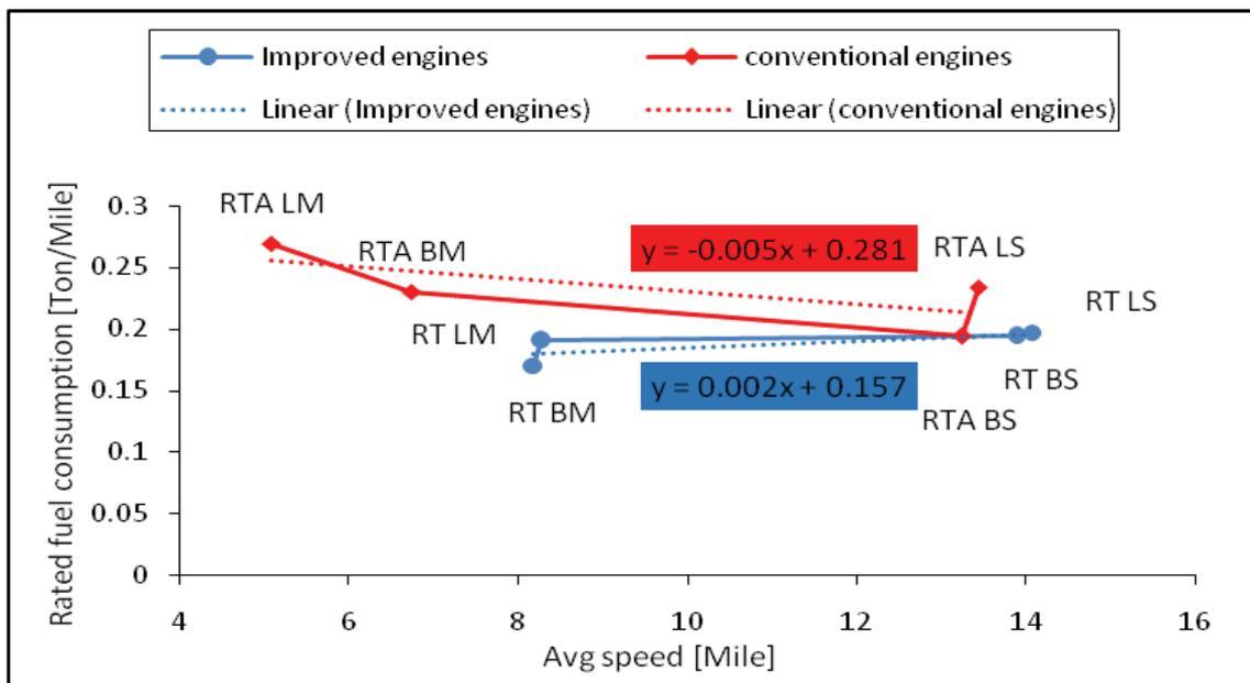
**Figure 14.** The rated fuel consumption for the conventional and improved engines; LM (load and maneuvering), BM (Ballast and maneuvering), LS (Load and steaming), and BS (Ballast and steaming)
