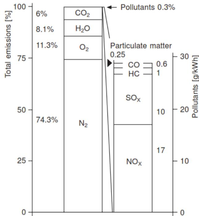
**Figure 15. Typical composition of the exhaust gas products of a diesel engine burning fuel (HFO) with an average 3% Sulphur content (Woodyard, 2004)**
