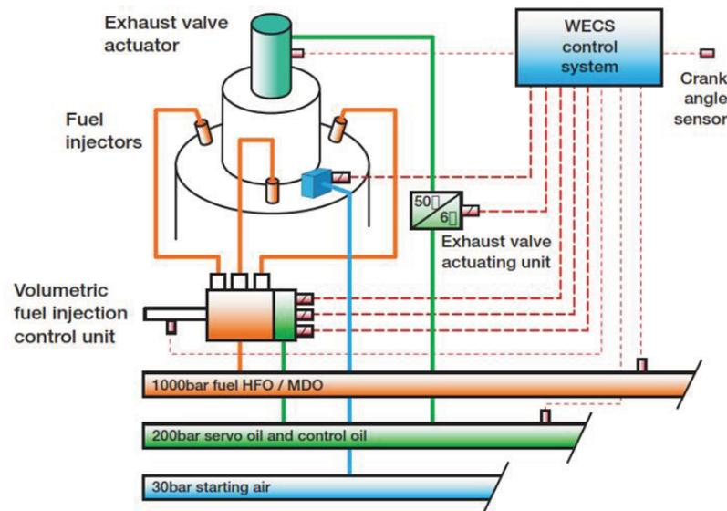
**Figure 5. Schematic of the common-rail systems in Sulzer RT-flex engines (Wärtsilä, 2004)**
