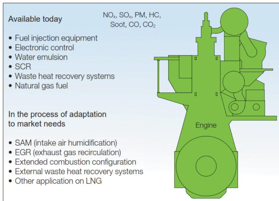
**Figure 3. Emission reduction methods (Emission Control MAN B&W Two-stroke Diesel Engines)**
