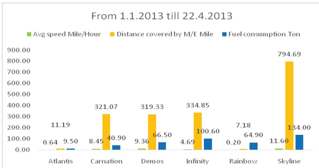
**Figure 10. NITC supertankers main engine fuel consumption (Sulzer RT-82flex) in ballast and maneuvering condition**
