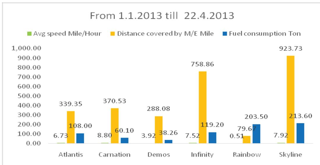
**Figure 11. NITC supertankers main engine fuel consumption (Sulzer RT-82flex) in full load and maneuvering condition**
