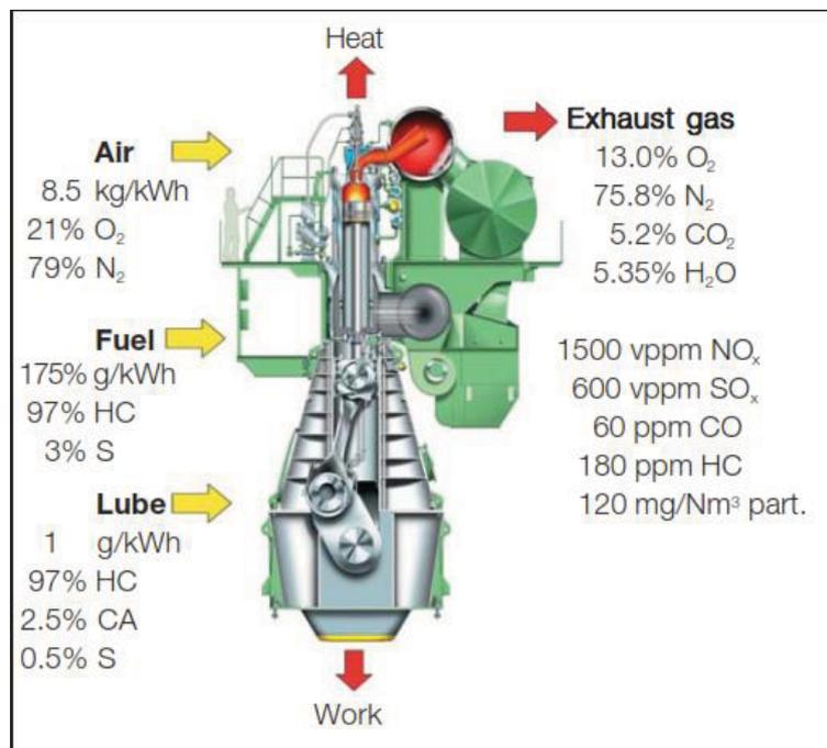
**Figure 1. Input and output of a typical two stroke diesel engines (Emission Control MAN B&W Two-stroke Diesel Engines)**
