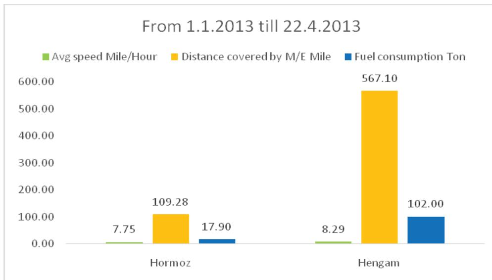
**Figure 6. NITC supertankers main engine fuel consumption (Sulzer 7RTA84) in ballast and maneuvering condition**
