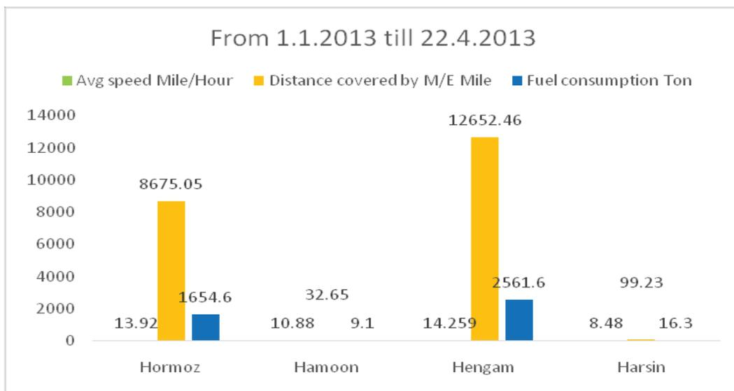
**Figure 9. NITC supertankers main engine fuel consumption (Sulzer 7RTA84) in full load and full steaming condition**
