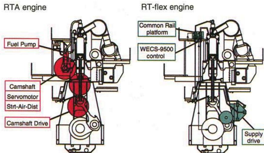
**Figure 4. Schematic of the conventional (RTA) and improved (RT-flex) engines**
